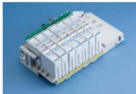
TDX Replaceable Module backplane fully removed
